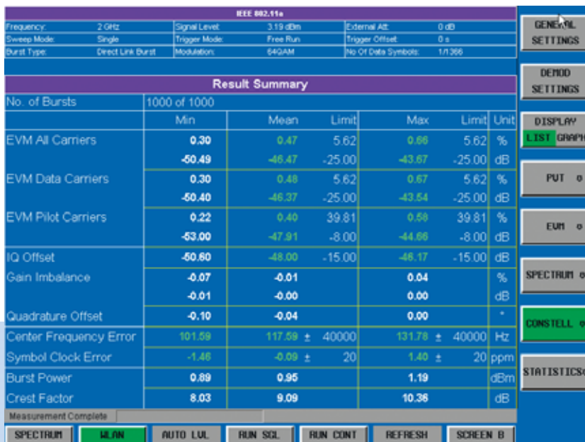
FIG 2: Display of the main modulation parameters in the Result Summary: The measurement covering 20 bursts shows an EVM of -46.7 dB for the best burst (min. peak) and -45.09 dB for the worst burst (max. peak) as well as an average EVM of -46.09 dB for all bursts. Output power (with regard to burst) and crest factor are also displayed. Quick and easy determination, for example, of the EVM dependence on the output power of an amplifier is thus possible. Owing to its auto level function, the analyzer follows these level changes without requiring any manual settings.
